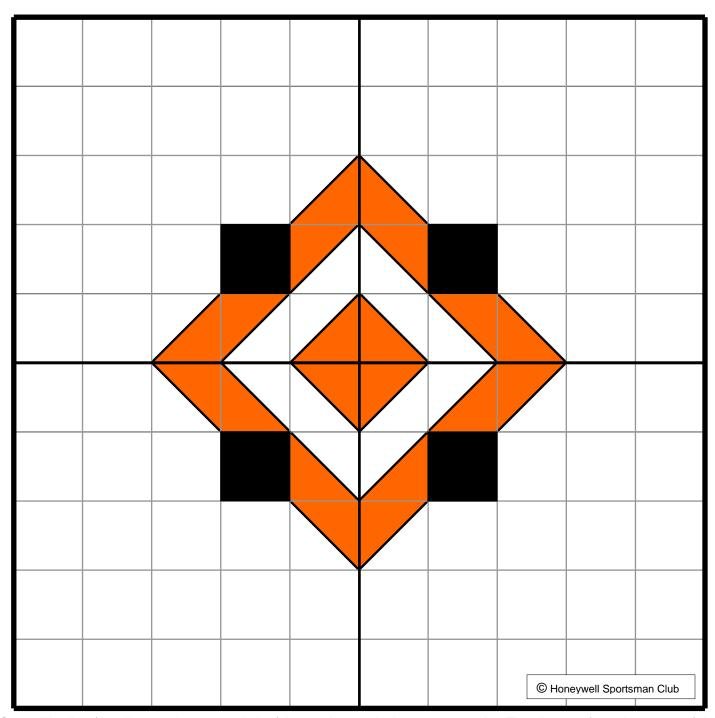
One milliradian (the distance between mil-dots) is equal to 3.6 inches at 100 yards. The distance from the center of the target to the edges of the large square is 3.6 inches in all four directions. The points of the diamonds are spaced at .2, .4, and .6 milliradian intervals, assuming the target is at 100 yards. At 50 yards, the diamond points are at .4, .8, and 1.2 milliradian intervals, with the target edge at 2 milliradians. The grid is at 2/10 milliradian intervals at 100 yards.
